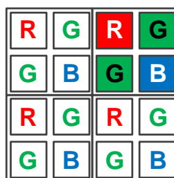
Figure 8-49 Horizontal and vertical color Binning by 2x2
