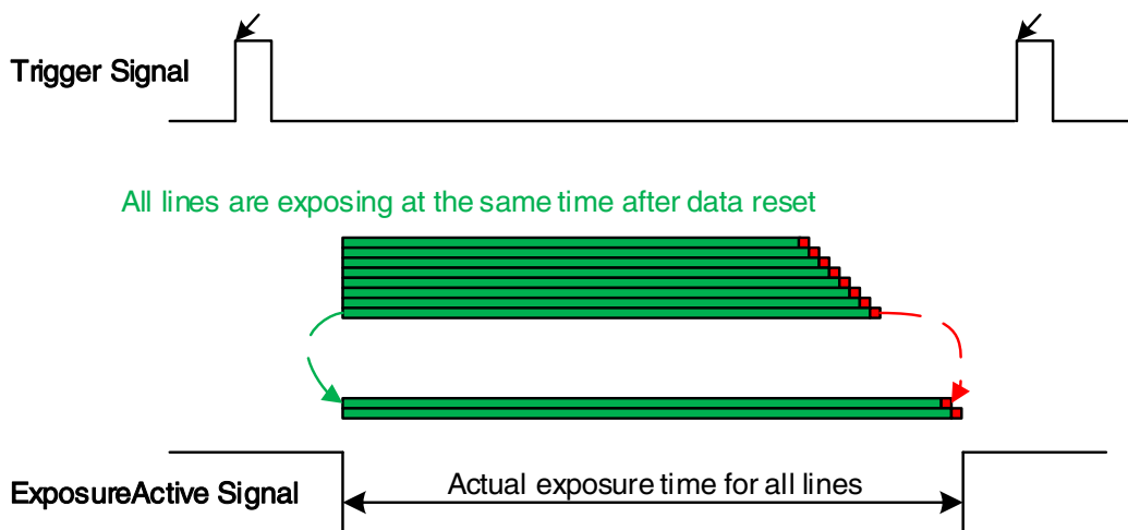
Figure 8-8 Global reset release shutter mode "ExposureActive" signal schematic diagram
